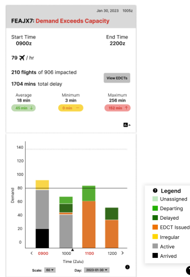
Figure 10: FSM graph of FCAJX7 showing demand exceeds capacity. Times where demand exceeds capacity are in red for greater salience.
